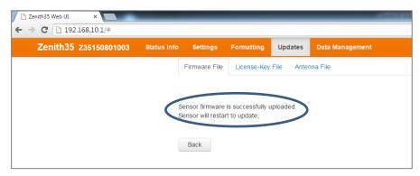
Please re-connect the receiver to the GeoMax Z35WebManager. The new firmware version should be displayed in the Hardware Info panel. To check please refer to chapter 3.6.1 "Checking the receiver firmware version".
