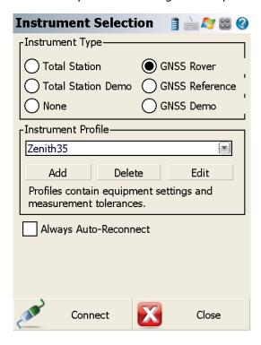
To ensure that measured heights are computed correctly, it is important to define the receiver type. At the *Antenna Height* panel, choose the Model as **Zenith35**. The Measured Height is the default length of the telescopic pole.
