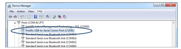
The COM Port defaults are Baudrate 115`200, 8 databits, 1 Stopbit, Parity None.
