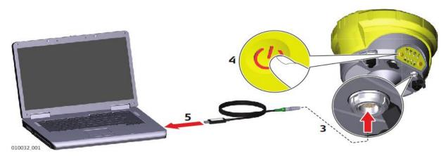
After the successful installation your hardware can be used as a mass storage device. Files can now be uploaded and/or downloaded to the Zenith35.
